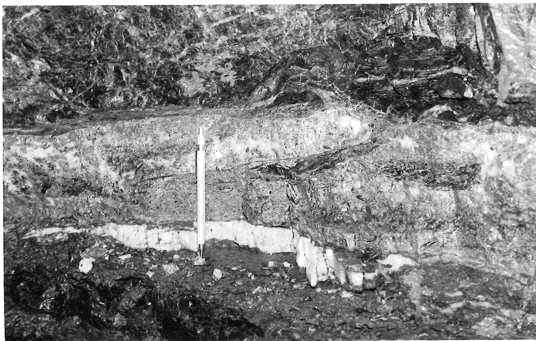
Figure 4: White unmineralised ribboned veins beneath a well-mineralised section of the Elandshoogte Reef, Elandshoogte Mine.
